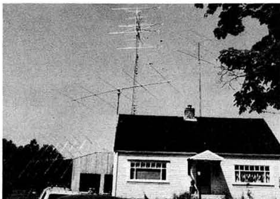
The vhf/uhf antenna farm of Dave Olean, K1WHS, in East Lebanon, Maine, USA. On the left may be seen the 336-element 144MHz moonbounce array, made up of 24 14-element Yagis. The three towers which can be seen over the rooftop hold, l to r: five-element Yagi for 28MHz; 144 and 432MHz terrestrial arrays; and 220MHz array and 50MHz Yagi. Photo: Nadine White
